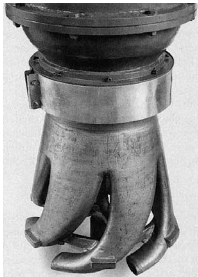
Prototype of a water turbine built according to EULER's proposals
